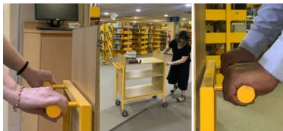
Figure 4. Load thrust with 4-wheel auxiliary equipment
