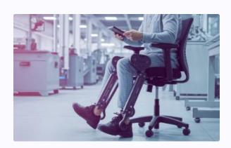
The Chairless Chair allows workers to alternate between sitting, standing, and walking without requiring a physical chair. This passive device locks into position when activated, creating a supportive structure that reduces fatigue during prolonged standing.
