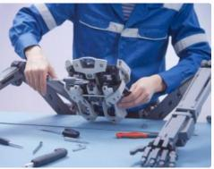
Taking apart the exoskeleton for storage, cleaning, or transport. This involves disconnecting components, organizing parts, and preparing for future use or storage.
