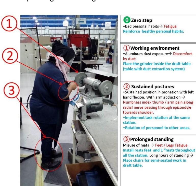
Figure # 9. Work center #30 deburring process.
