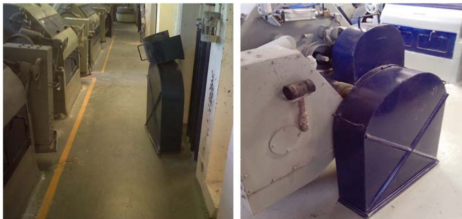
Figure 8. Placing safety guard in machinery
