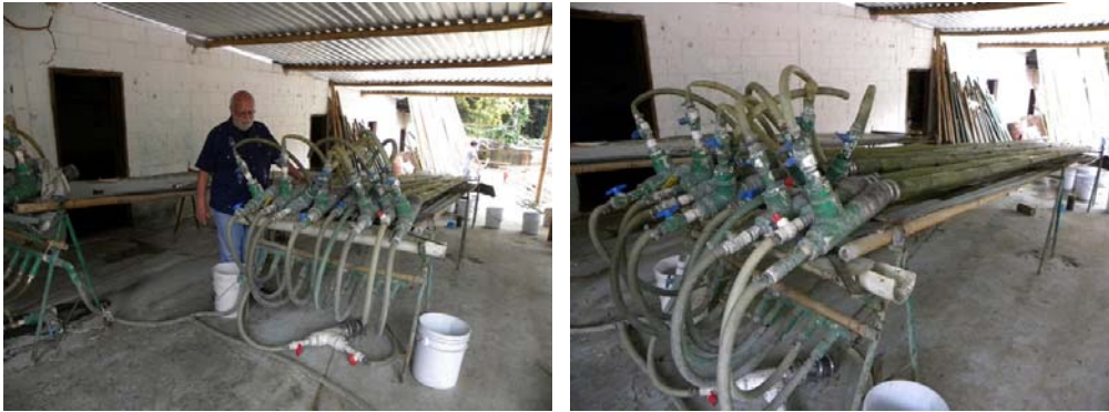
Figure 1. Preservation of bamboo poles by modified Boucherie technique.
