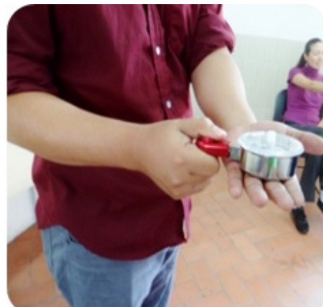
2.-How to property hold the dynamometer for the pinch effort
