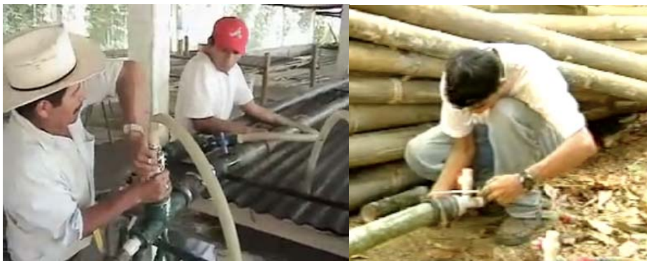
Figure 2 Fixing the clamps embracing the culm end.
