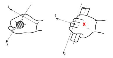
Figure 2: Coordinates system for the measuring of the vibrations transmitted to the hands.
