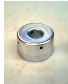
Figure 3.3. Original hand tool made of galvanized sheet metal
